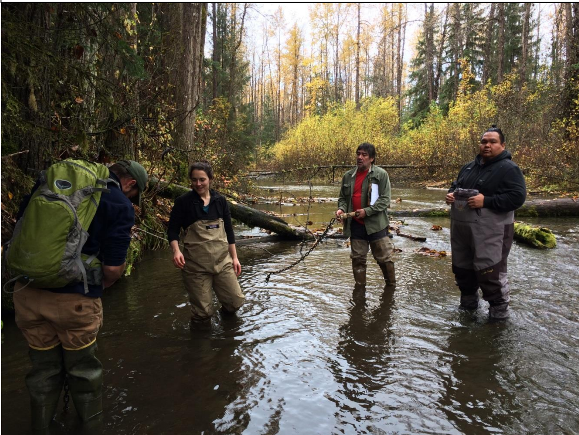
Figure 1. SAWC Science Director working with members of the Chilkat Indian Village to install a stream temperature data logger, September 2017.
